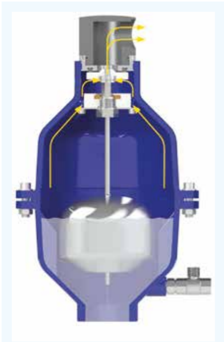
Air release during working conditions
